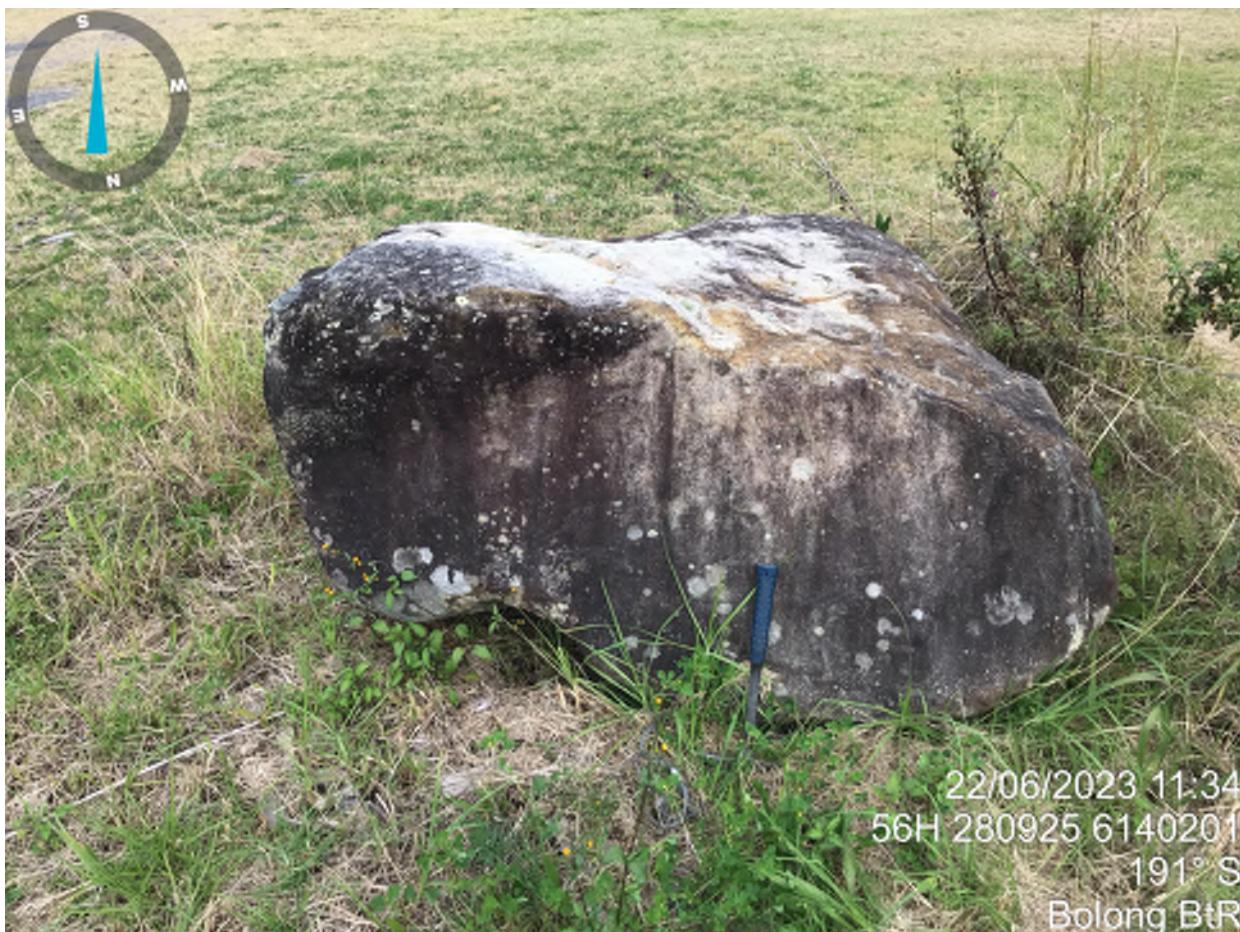
PHOTO P8 - ROCK FILL FLOATER OF HIGHLY TO MODERATLY WEATHERED SANDSTONE MEDIUM TO HIGH STRENGTH
